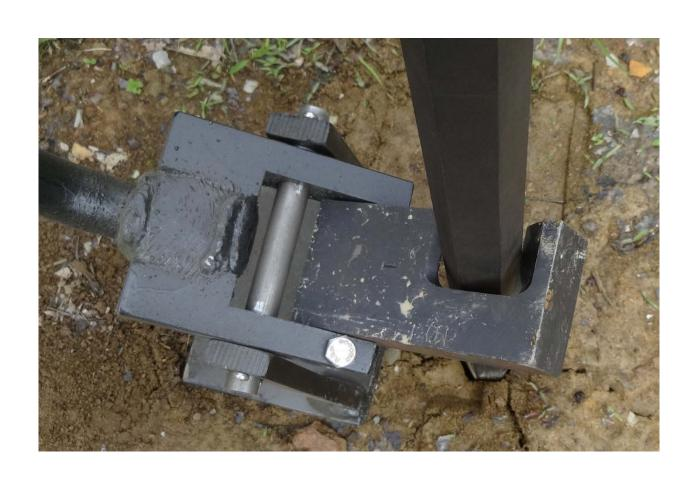
The bar puller handle must be close to the probe bar after attaching the bar puller block onto the probe bar.
