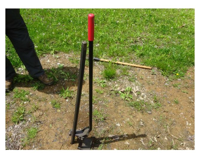
Block is properly attached on the flats of the probe bar.
