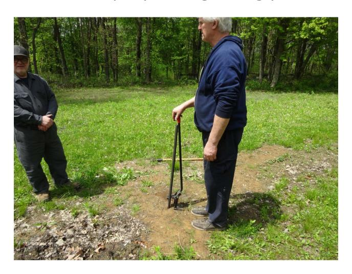
Handle strokes beside and slightly behind the operator. Block moves probe bar upward out of the ground.
